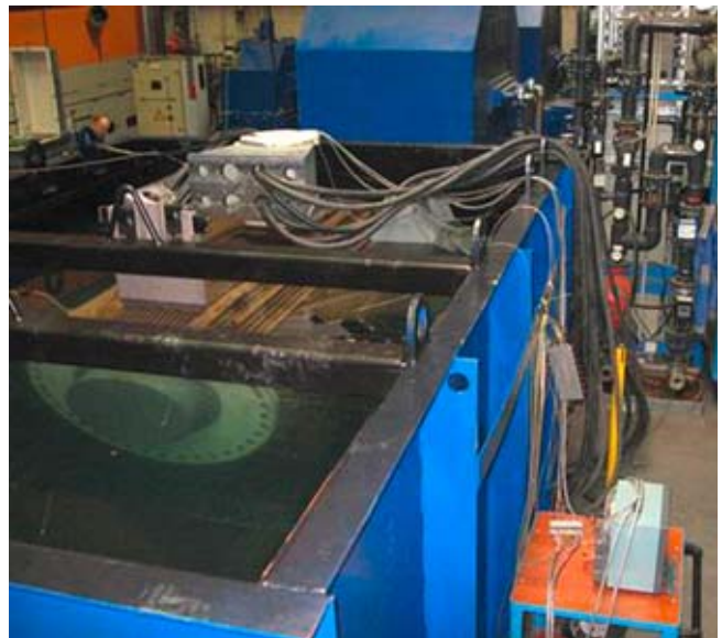
Ruhstorf test facility – water basin for submersed heat run test up to approx. 3 MW
