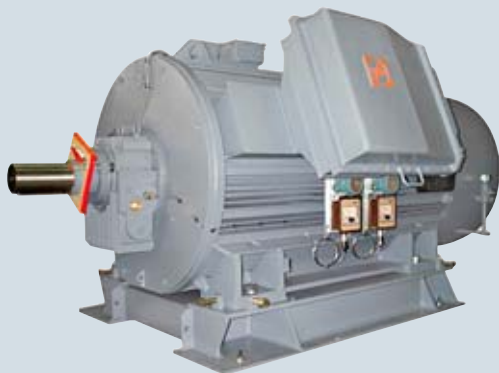
Retrofit example: LOHER VARIO Rib-cooled motor with base frame plate for height adaption, shaft modification and terminal box adaption (non-flameproof design)
