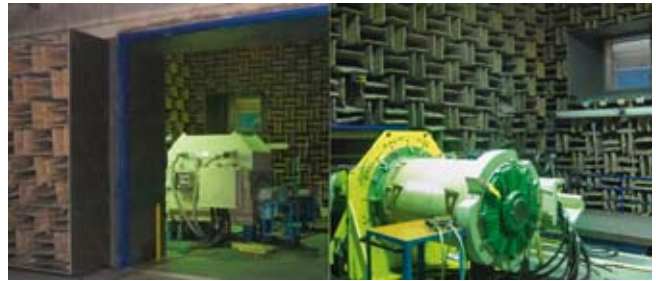
Ruhstorf test facility – noise test room for measurements at load condition
