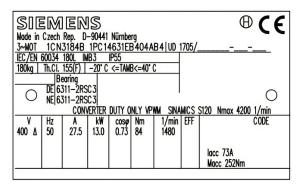
1PC1463 - steel plant motor for converter operation, naturally cooled without external fan, enclosed version
