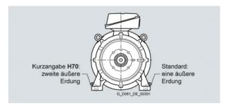
Design of the terminal box for steel plant motors
