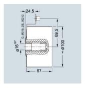
Mounting dimensions of LL 861 900 220 rotary pulse encoder
