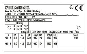
1PC1443 - steel plant motor for converter operation, self-ventilated
