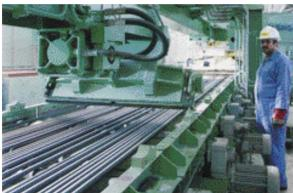
Steel plant motors - transport material for coiling
