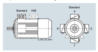
Location of the terminal box with the corresponding digits in the 16th position of the Article No.
