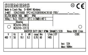
1PC1423 - roller-table motor for converter operation on the SINAMICS S120
