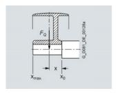
In order to calculate the admissible cantilever forces for a radial load, the line of force (i.e. the centerline of the pulley) of the cantilever force  $F_{\rm Q}$  (N) must lie within the free shaft extension (dimension x).
