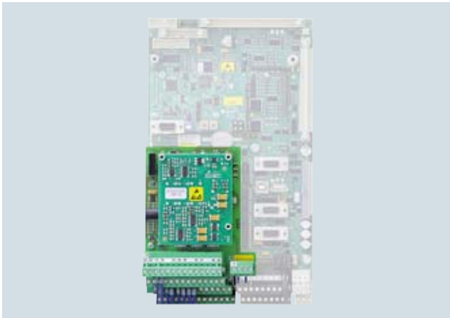
G05 Peripheral board 4 in the cabinet unit
