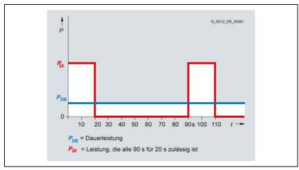
Fig. 8-4 Load diagram
