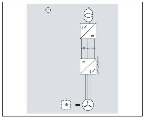
Fig. 5-4 Basic circuit
