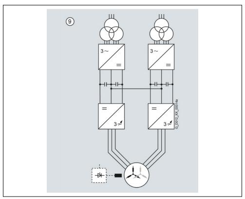
Fig. 3-6 Increased power rating by connecting two converter units in parallel <sup>1)</sup>, 24-pulse infeed
