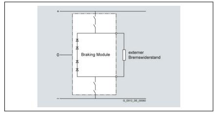
Fig. 8-3 Block diagram, Braking Module with braking resistor
