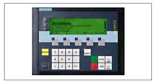
The AOP30 operator panel is fitted into the cabinet door of the SINAMICS GM150 to enable operation, monitoring and commissioning.
