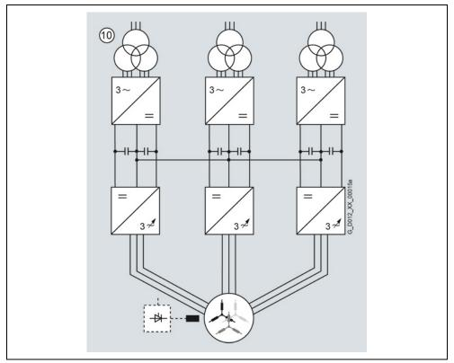
Fig. 3-7 Increased power rating by connecting three converter units in parallel <sup>1)</sup>, 36-pulse infeed
