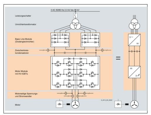
Fig. 2-3 Block diagram
