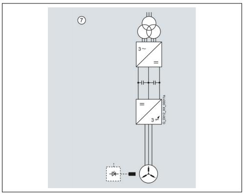
Fig. 3-4 Basic circuit, 12-pulse infeed
