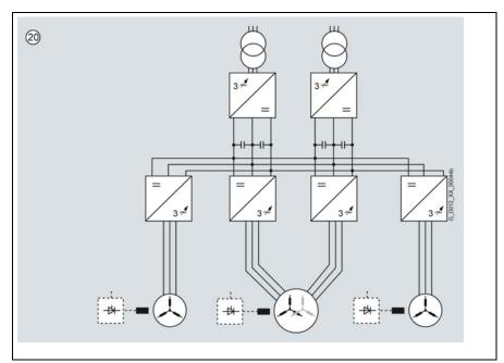
Fig. 6-13 DC bus configuration with two Active Line Modules and three motors connected to a common DC link (2 × 10 MVA, 1 × 20 MVA)
