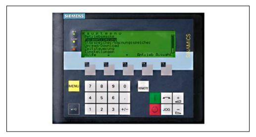
The AOP30 operator panel is fitted into the cabinet door of the SINAMICS GM150 for operation, monitoring and commissioning.
