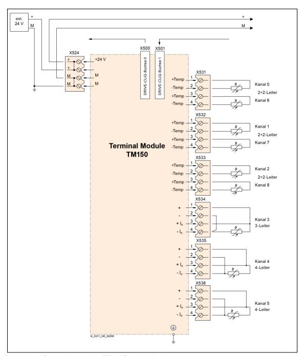
Fig. 8-1 Connection example, TM150 Terminal Module
